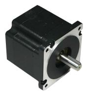
The 34Y112S-LW8-MS High Torque Stepper Motor offers a great value without sacrificing quality. This motor was designed to offer the highest possible torque while minimizing vibration and audible noise. It is wired in series with a Molex 4 pin Mini-Fit Jr. receptacle.
