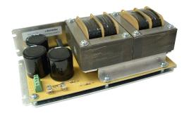
The PSA80V4A-1 power supply has a single 80V output, a voltage input of 115 or 220VAC, and power capabilities of up to 320 watts. With an unregulated output and a size of 8.30" x 4.25" x 2.81" and dual mounting position "L Bracket," the PSA80V4A-1 can be mounted just about anywhere. The PKG-341-MBC08-PS-CBL includes two wires for powering the MBC12101.
